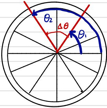
$$\omega_z = \frac{d\theta}{dt}, \quad \alpha_z = \frac{d\omega_z}{dt} = \frac{d^2\theta}{dt^2}$$
