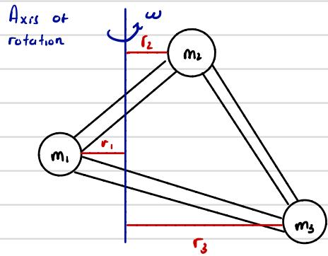
$$I = \sum_i m_i r_i^2 = m_1 r_1^2 + m_2 r_2^2 + \dots$$
